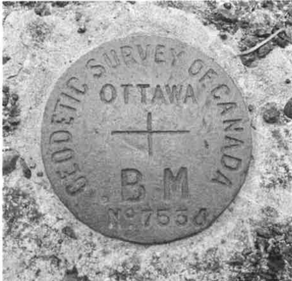
Figure A6-4. A geodetic survey benchmark.
