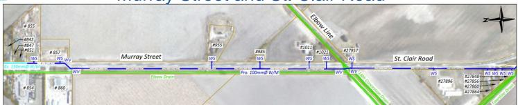
2,702 meters of 100mm diameter watermain with water service connections to properties. This watermain would be installed by open-cut and directional drilling method.
