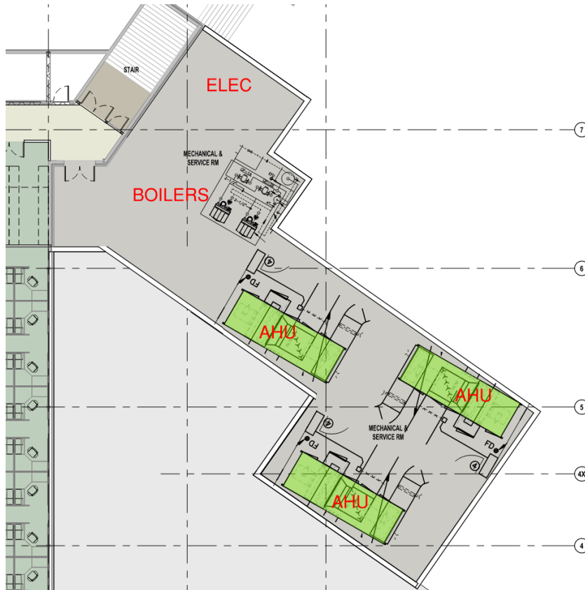
Floorplan Sketch 2 : Museum AHU-Boilers and Main Elec Service in New Penthouse Area
